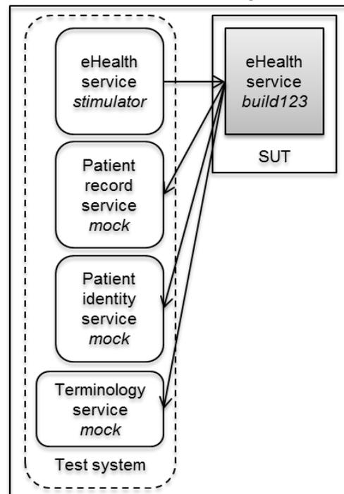
Figure 5. Test environment for non-terminal service unit test.
